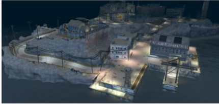
Figure 1: Inferred lighting allows this complex scene with 213 active lights to be rendered at 1280x720 resolution, with 8x MSAA, at 23fps (4:3) on a GeForce 8800GTX.
