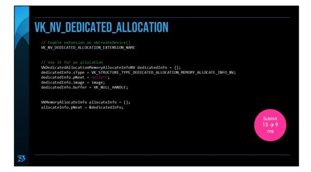
"Normal device memory allocations must support memory aliasing and sparsebinding, which could interfere with optimizations like framebuffercompression or efficient page table usage."
